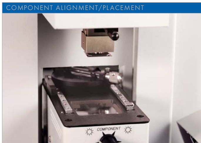
PBGA being held by Vacuum pik during Alignment procedure
