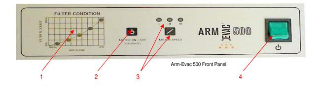
The Arm-Evac 500 has a graphical Filter Condition Display (1) which continuously monitors filter condition. As the system filter(s) collect particulates, LED's on the Filter Condition Display will illuminate along the graphical curve of the display.
