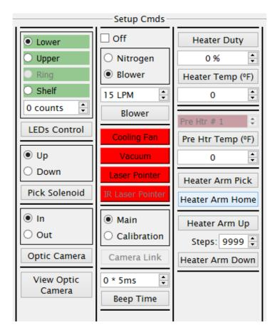
To the left is the Setup Commands portion of the Debug screen. Each box deals with activating a different aspect of the TF-1800 machine. The user can select or change options, then press the associated button in the box to implement the changes.
