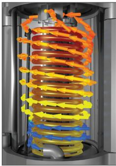
Inductive-Convection Heater pre-heats the air in a cyclonic fashion around the induction coil before it enters the inner chamber.
