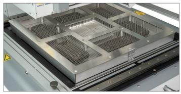
Powerful IR Preheater allows for fast, efficient bottom-side heating and is height adjustable to provide more aggressive thermal transfer on higher mass PCBs (TF2800 shown).
