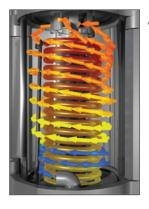
Heater pre-heats the air in a cyclonic fashion around the induction coil before it enters the inner chamber.
