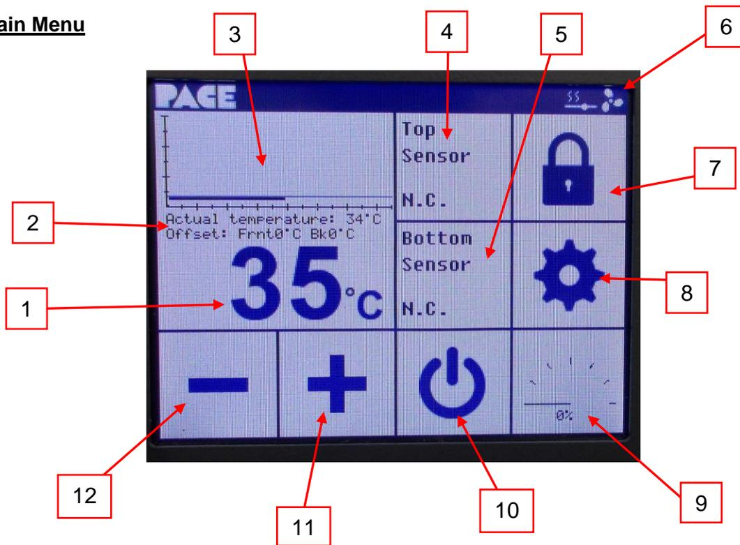
1. **Set Temperature:** Set the temperature by tapping the number. A numeric keyboard will appear that will allow you to set the temperature from 20 - 200°C (68 - 392°F). Temperature can also be set by tapping the + or - buttons.
