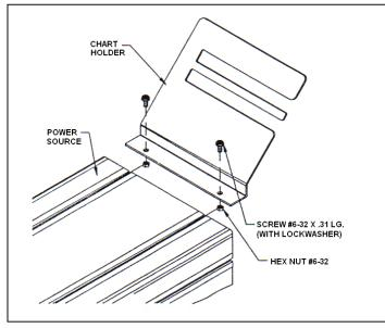
3. Install the Tip & Temperature Selection System Charts (in booklet form) onto the Chart Holder Assembly by sliding the metal spiral ring which binds the charts onto the metal finger of the Chart Holder Assembly. Refer to the illustration to the right.
