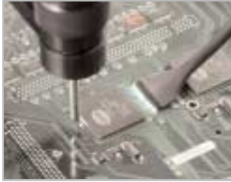
The LS 3000 Rigid-Probe with back lighting inspecting a PBGA
