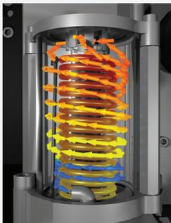
The **Inductive Convection Heater** pre-heats the air in a cyclonic fashion around the induction coil before entering the inner chamber, where the air is instantly heated to the target temperature. The low thermal mass design then allows the coil to cool down at a faster rate, consistently yielding high quality solder joints.
